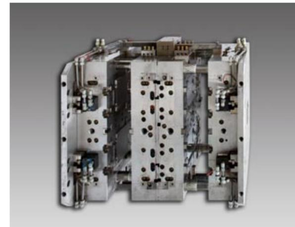
**2+2 Stack Mold:** Design technology; highly accurate fabrication technology, craftsman-grade finishing; molding technology (Industrial Industry)
