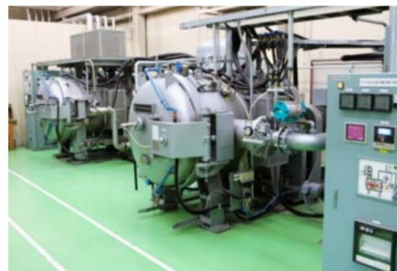
**Vacuum thermal processing equipment:** Critical to maximizing the metallic properties of our molds is maintaining vacuum quenching (quick cooling) conditions suitable for the raw materials used for a given mold component. To understand these conditions, we have established a vacuum quenching facility where we record data on quenching conditions for later use. With this system in place, we can apply our accumulated data and expertise to derive the best metallic properties for our molds.
