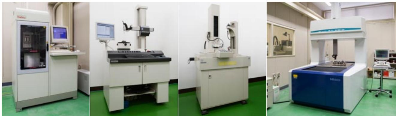
From left: laser modeling system, roundness measuring instrument, gear measuring instrument, 3D measuring instrument
