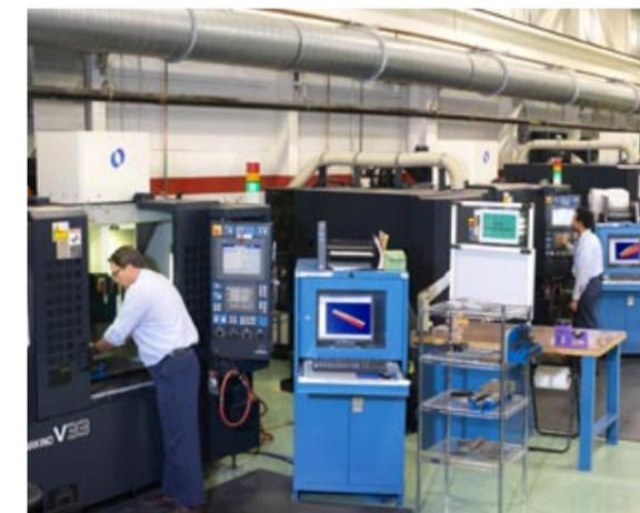
**Mold Shop:** Our mold shop factory boasts a bright, spotless environment and features top-end fabrication equipment. Accurate, high-quality metal molds cannot be manufactured without constant temperature and humidity conditions. Maintaining these conditions is so imperative we cannot stop the factory's air-conditioning system even when the plant is closed for a holiday.
