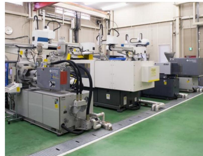
**Injection molding equipment for trial runs:** Our customers' precision specifications cover not only the dimensional accuracy of the mold components but also the dimensional accuracy of the molded parts. Having the ability to test these data sets against each other makes it possible to quickly determine any compensation or correction values that may be required. Canon manages a system designed to address our customers' rigorous dimensional specifications.
